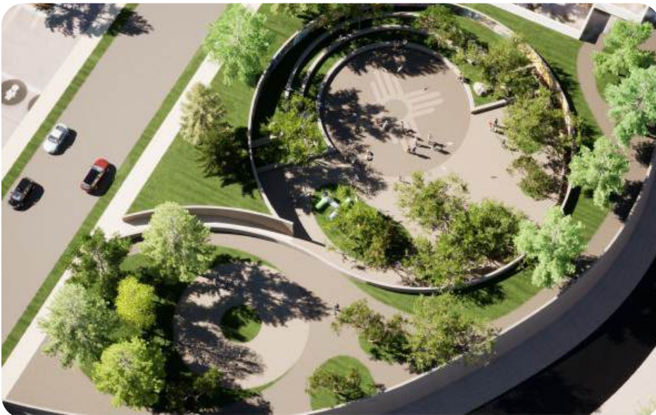
Figure 8.6 (A,B,C,D,E,F): A proposed stormwater retention basin concept repurposes an underutilized area to manage overflow during heavy rain events. The design integrates a circular basin for water capture with surrounding multi-use public space, including shaded plazas, walking loops, and playful areas that engage the community even during dry periods. The basin provides dual functionality with flood mitigation and civic activation.
