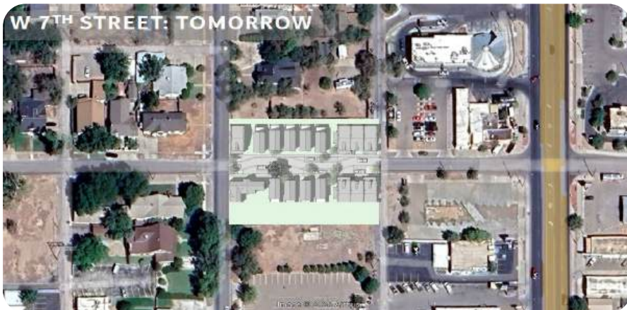
Figure 4.6 (A, B, C, D): Illustrate how W 7th Street can evolve from an underused corridor into a multi-functional public space: re-designing vehicle patterns, adding permeable green areas and integrated traffic calming measures transform the street into a safer, more flexible environment that supports stormwater management, pedestrian activity and community gathering.
